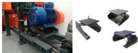
Motor Base used in Belt Drives to Maintain Optimal Belt Tension
