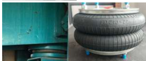
Air Bellow used in Continuous Casting Machine
