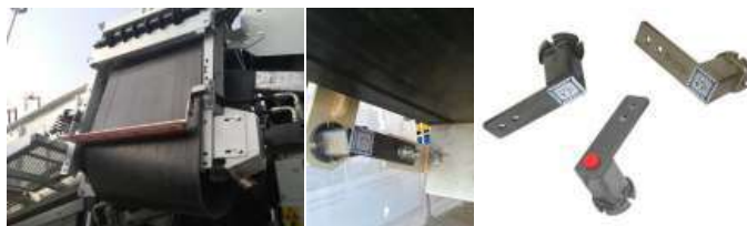
Tensioner Used in Belt Scrapers
